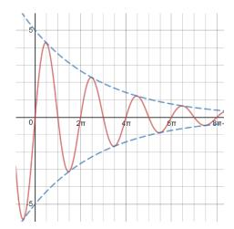
**Carrier Waves:** Another wave form can be the "envelope" for a oscillations! These is how music on the radio is "carried", by a sinusoidal "envelope" called a "carrier wave". This signal can be filtered out, then voila! You have just the actual waves that translate into music or talk or whatnot.
